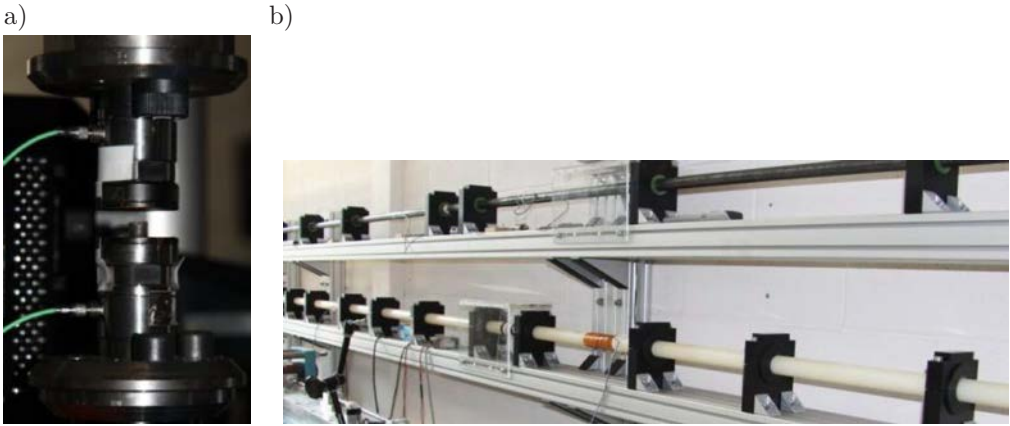
FIG. 2. a) VHS setup, b) Hopkinson bars setup.
