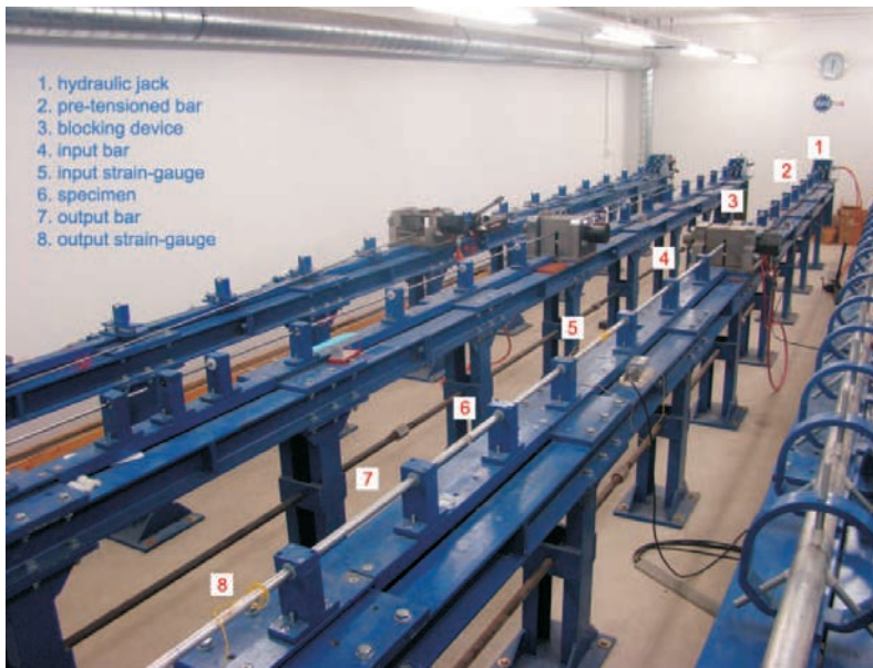
FIG. 3. High strain-rate tensile tests on specimen \varnothing = 20 mm.
