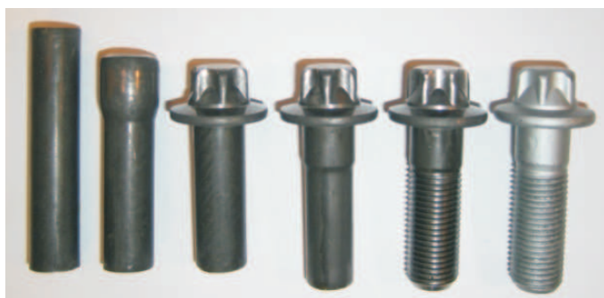
FIG. 2. Sequence of cold forming of fastener.
