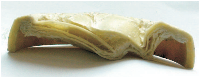
FIG. 12. Cross-section of the destroyed sphere shows delamination of the plays.
